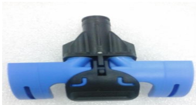
Figure 4. A device that absorbs short fibers
