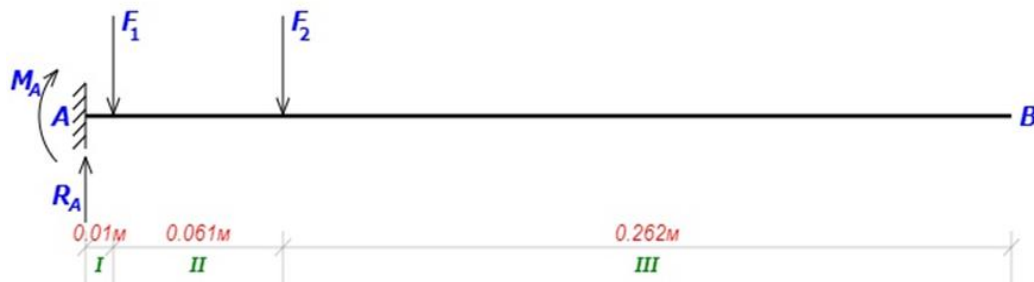
Figure 4.1. The calculation scheme of the cantilever installation of the exchanger element on the column
