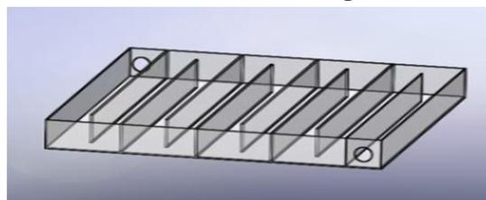
Fig. 1.a. Scheme of the collector channel box.
