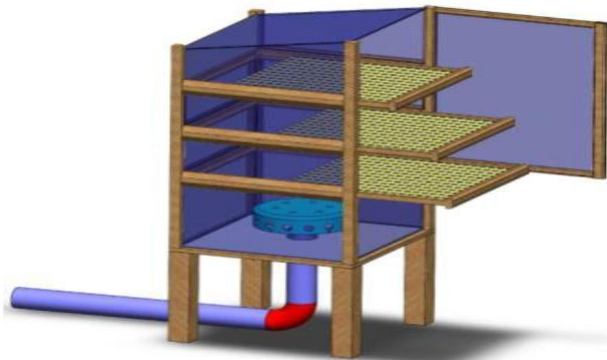
Fig. 1. b. Scheme of a greenhouse-type dryer
