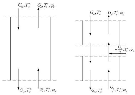
Calculation scheme for a cooling tower with one air supply. cooling towers supplied with intermediate air
