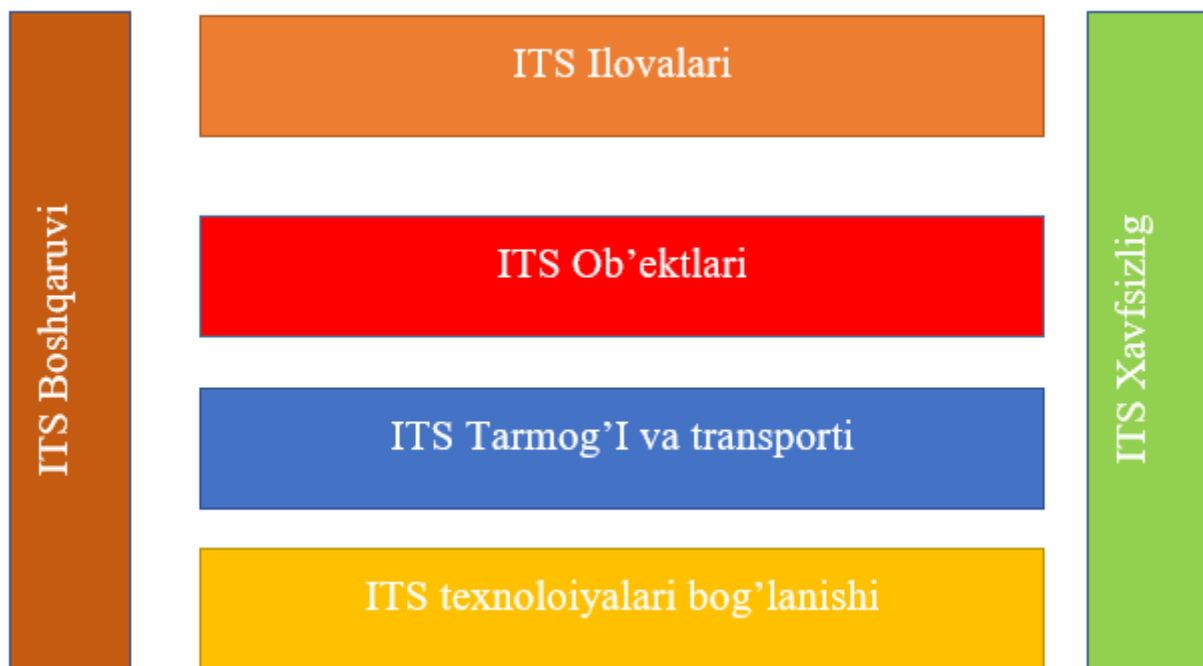
2-rasm. ITS aloqa protokollari to‘plami
