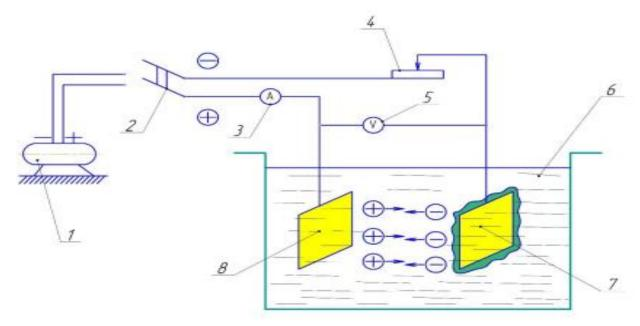
Figure 1: Schematic view of the electrolysis process: anions; -cations;
