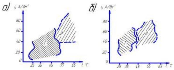
Figure 2. Hard surface (T) and wear-resistant (I) chrome plating. a) CrO3 - 150 g / 1 concentration b) CrO3 - 250 g / 1 concentration.
