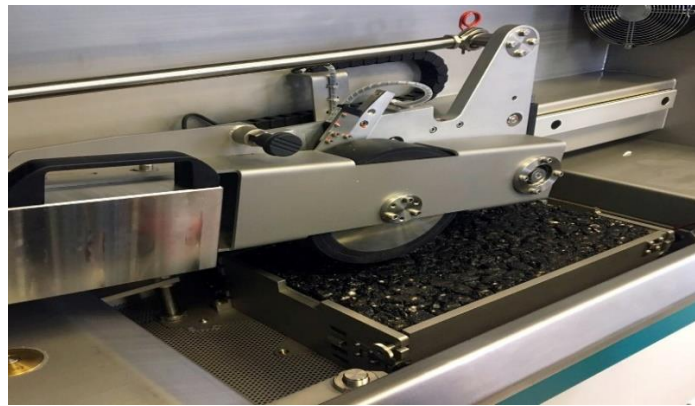
Fig. 3. A device for testing asphalt concrete pavements for rutting.
