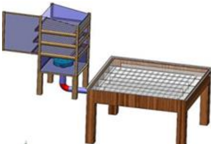
Fig. 1.s. The scheme of the solar cell is a collector combined with a dryer.
